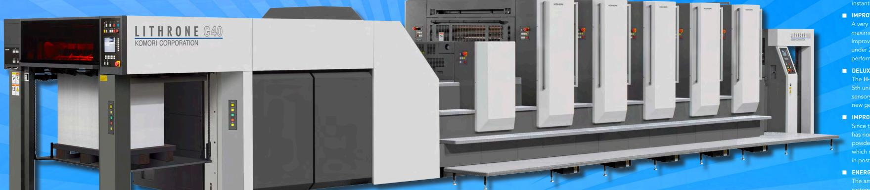
Perhaps the best innovation is that the **H-UV** system ensures that print jobs (even on substrates) can be cut and folded <u>immediately</u> after printing. This eliminates the need to leave work standing for hours before being dry enough to process.
